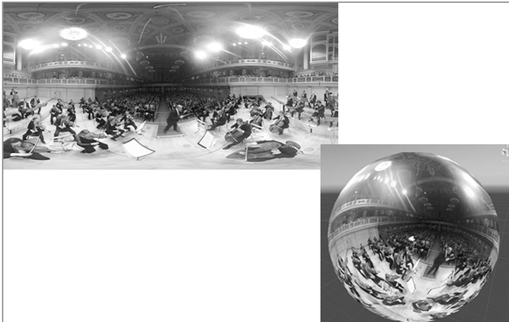
Fig. 4. Distorted video and projected video inside a sphere
