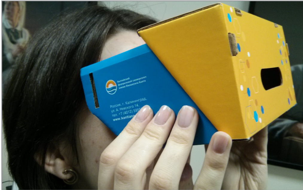
Fig. 5. Viewing the spherical stereoscopic image with the help of the smartphone and stereoscope
