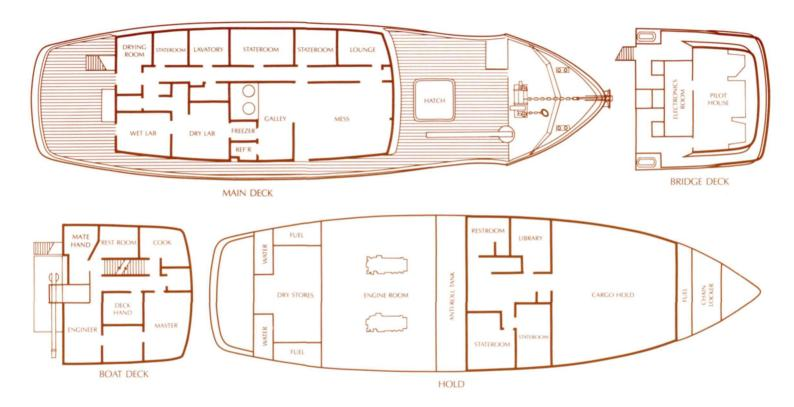
The *Tiĝla*x̂ is outfitted to conduct scientific work at sea. Wet and dry laboratories are provided for examining and preparing specimens which can be stored in special freezers. Depth sounders, water sampling devices, sonar, salinity and dissolved oxygen sensors, sampling nets, and data processing equipment are available to collect data on the physical properties and inhabitants of the sea.
