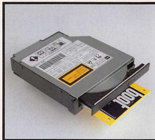
TWO MINTS IN ONE Check it out. The 1.44MB floppy and 11x CD-ROM are combined in a compact, unit. Very cool.
