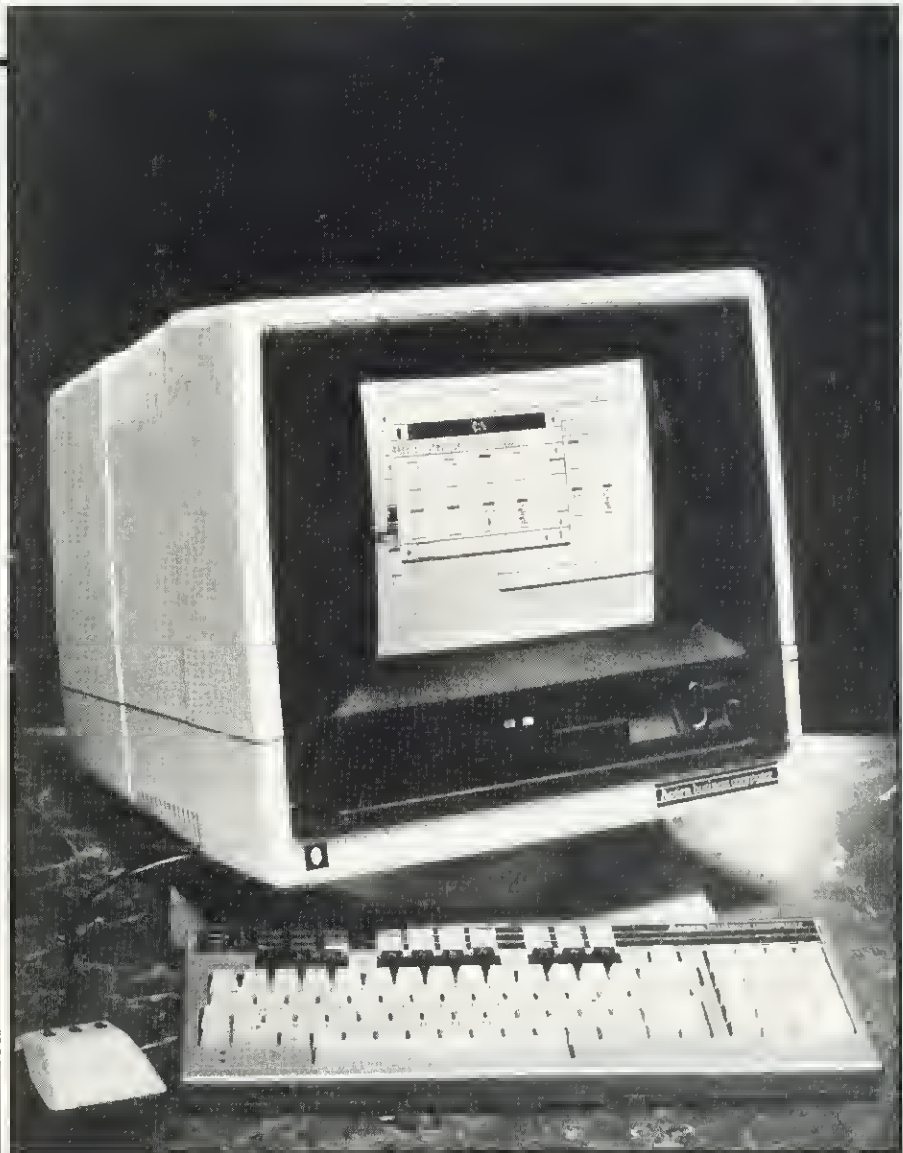
A marvel on marble: the ABC310 in all its glory. Beneath the monitor screen on the left is the Winchester hard disc, with the floppy drive beside it. Note the new symbols on the keyboard, re-arranged function keys, keypad and the mouse. There is no break key, but a reset is fitted on the rear of the keyboard. The monitor can be tilted and swivelled on its stand
