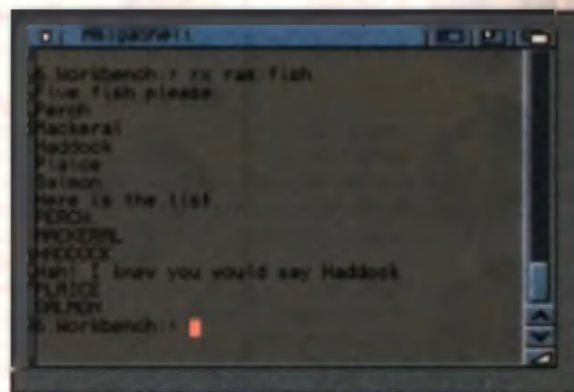
▲ Figure 3: compound variables are handy when it comes to dealing with lists of items which you want to store and maybe add to later.
