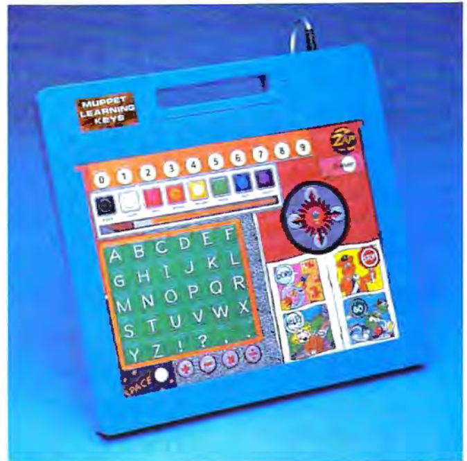
Koala Technologies' Muppet Learning Keys is an auxiliary computer keyboard especially suited for young children.
