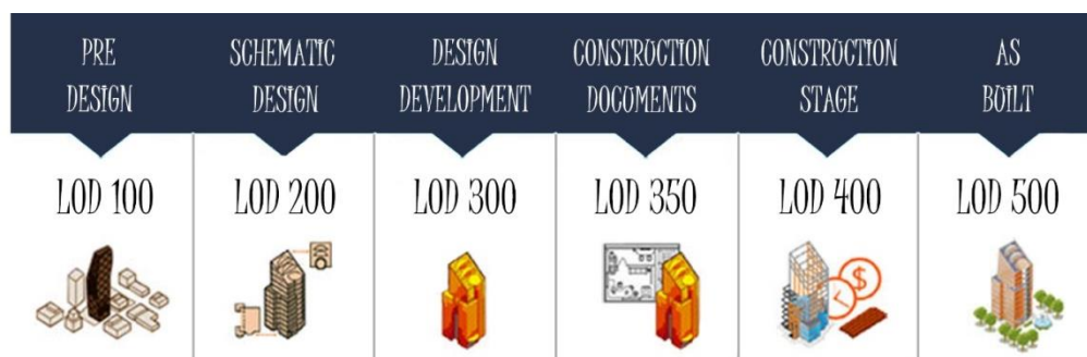
Figure 55: Descriptive diagram of the LOD concept
