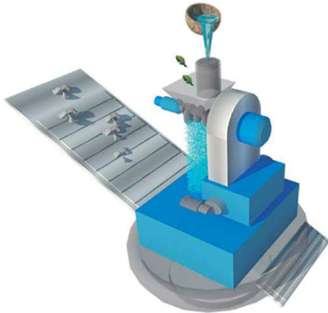
Figure 2. The biomachine Probila. Unit 3, where the sediment with gold is in contact with the Balsa extract, is highlighted.
