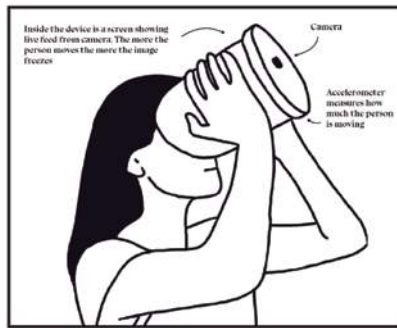
Figure 5. Description of Device's No.1 operation Figure 6. Prototyping and testing Device No.1
