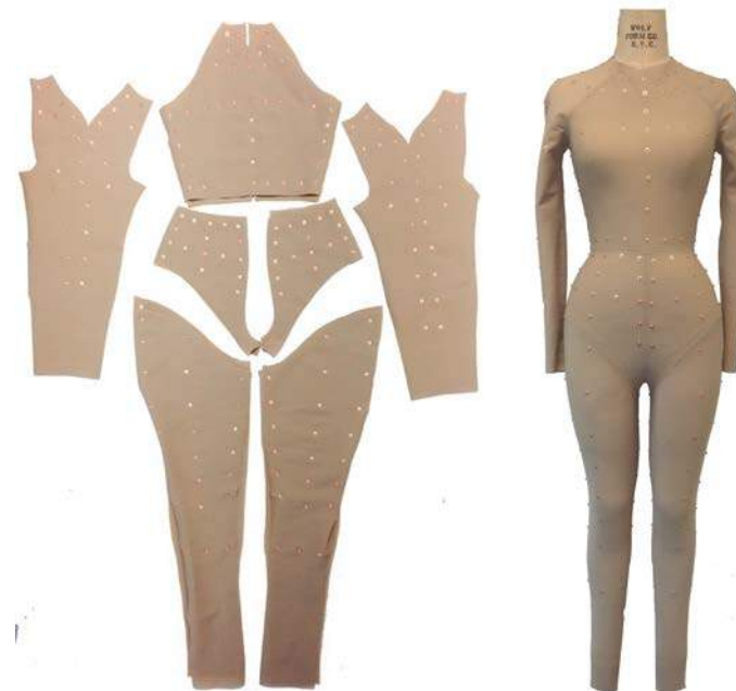
Figure 5a. Placement of the press-fasteners on the bodysuit before stitching Figure 5b. Positioning of the bodysuit as a completed piece.
