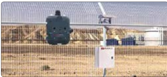
RoboGuard is a revolutionary agile scout robot, which runs along secured fences, ensuring perimeter integrity and capable of responding promptly to intrusion alerts. It consists of an autonomous unit, travelling on a monorail and carrying several sensors. (photo credits: magal)
