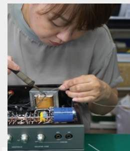
Soldering in a transformer. Every single solder joint in an Air Tight product is done by hand.
