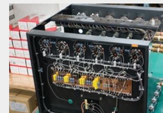
An ATM-2001 Reference in the process of being built. Note the point-to-point wiring.
