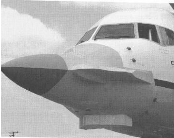
A close-up view of the F-22 forward fuselage attached to the Boeing 757 FTB. The 757 FTB (N757A) is the first 757 built. Boeing installed the sensor wing in late 1998. ( The Boeing Company. )
