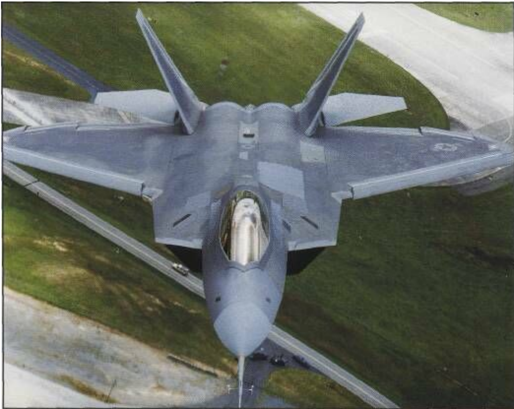
Raptor 02 departs Dobbins ARB on June 29, 1998 for its first flight. The shape of the F-22 perhaps contributes to the most important part of its stealth capability. ( Lockheed Martin Corporation. )
