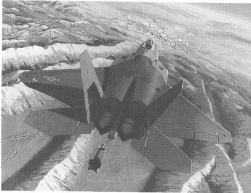
From about 15 mi away, an F-22 sends one of its two GBU-32 JDAMs on its way toward a predetermined target. With a CEP of only about 6 m 234 in, the satellite-guided JDAM is an extremely lethal weapon. ( Lockheed Martin Corporation. )
