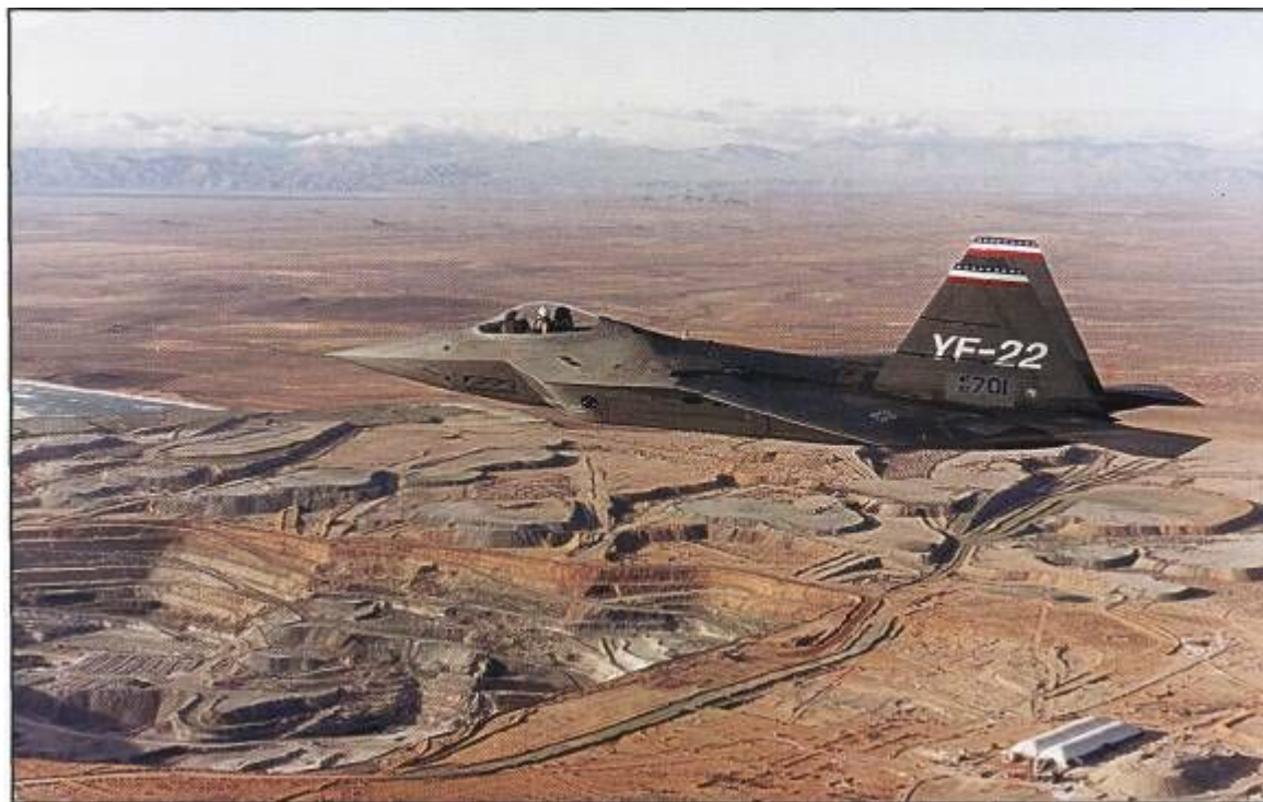
Powered by two Pratt & Whitney YF119-PW-100 prototype engines, the YF-22A prototype 2 (87-0701) flies near Edwards AFB. This is the airframe-powerplant combination that the USAF selected for what has now become the F-22A Raptor. The YF-22A's nose landing gear retracted aft while the F-22A's retracts forward. (Lockheed Martin Skunk Works.)
