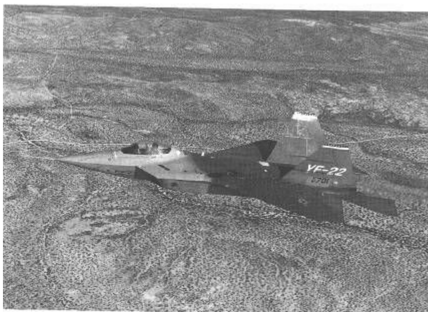
At 64 ft, 2 in long, the YF-22A is 4 in shorter than an F-15C. Their respective wing spans are nearly identical: 43 ft, 0 in versus 42 ft, 9% in. ( Lockheed Martin Corporation. )
