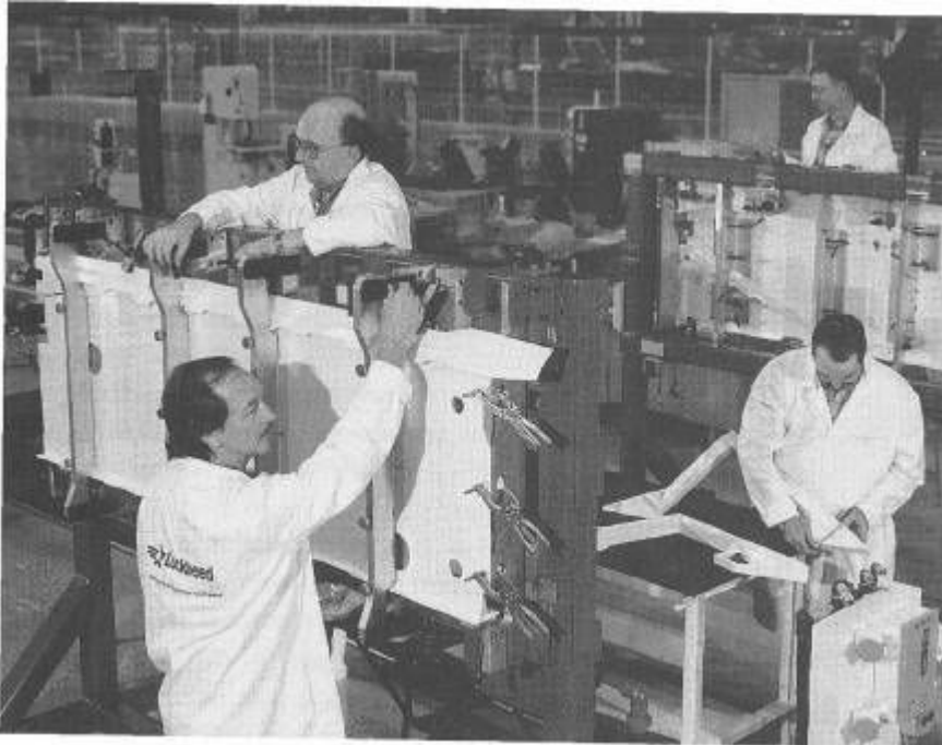
Beginning construction on Raptor 01 on November 2, 1995, LMAS employees Tommy Cole (left foreground) and L. D. Fleeman (left background) load the lower cap on to the nose landing gear wheelwell sidewall (known as a "web") while Dennis Watts (right foreground) checks one of the frames that will be attached to the web. Harold Morris (right background) is doing a preinstallation check on the other web. This was the first phase of building the first forward fuselage section. (Lockheed Martin Corporation.)
