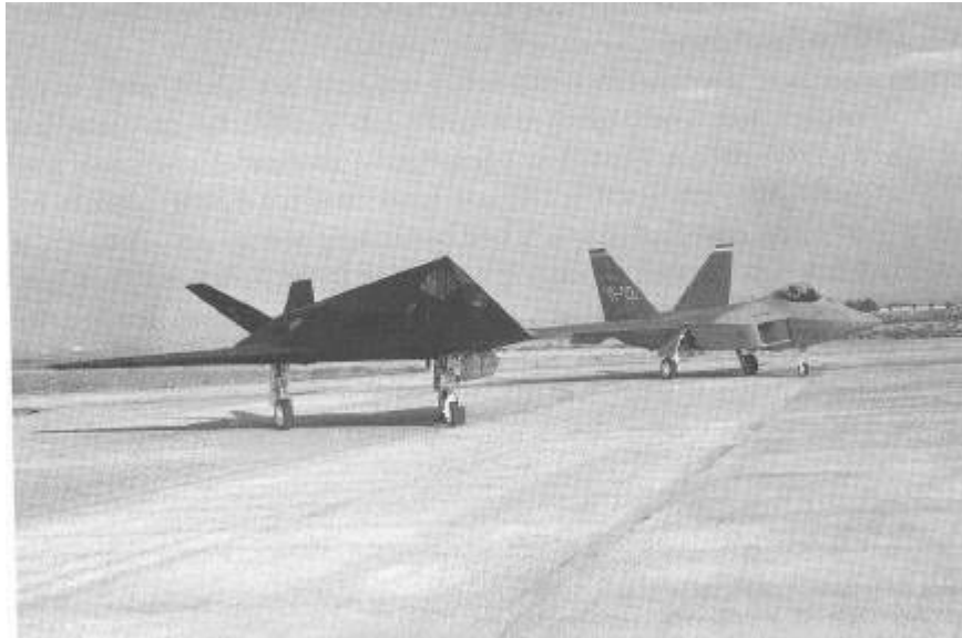
Evolution of stealth. In this rare photograph taken in January 1991, a Lockheed Martin F-117A Stealth Fighter, the world's first operational aircraft designed to exploit low-observable or stealth technology, poses with the P&W YF119-powered YF-22A ATF prototype. While the former was designed on a two-dimensional computer program, the latter was created on a computer with three-dimensional capability. (Lockheed Martin Corporation.)
