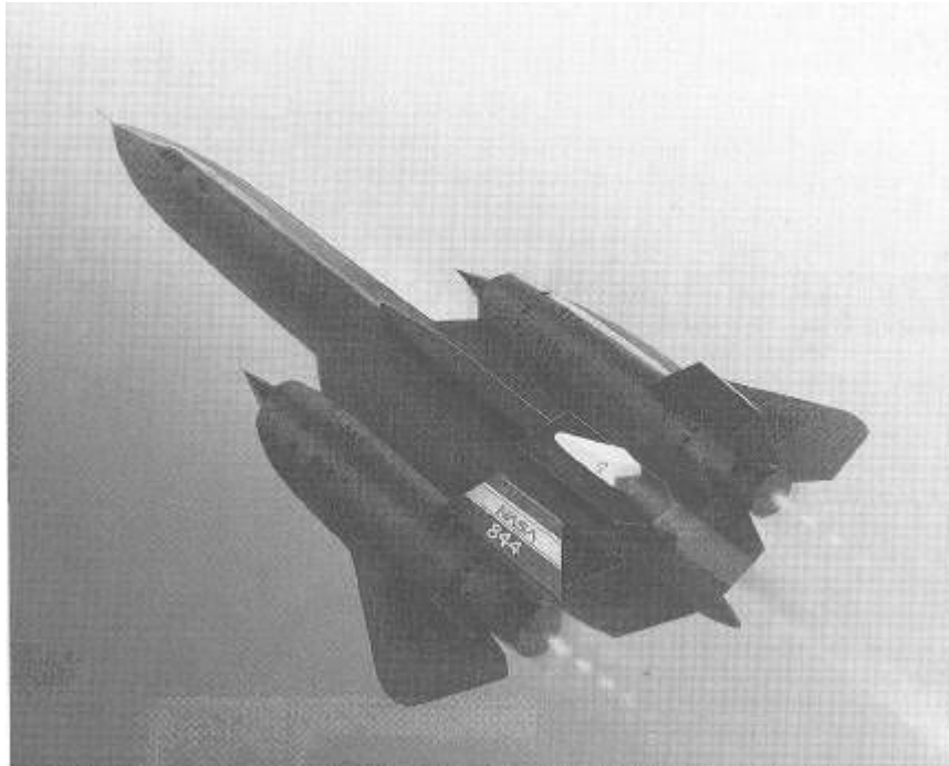
Considered the first-generation stealth aircraft, this artist's concept of an SR-71A Blackbird fully illustrates its wing-to-engine nacelles blending, fuselage chines, and inward-canted vertical tails, which all contribute to its stealth capabilities. ( Lockheed Martin Skunk Works. )
