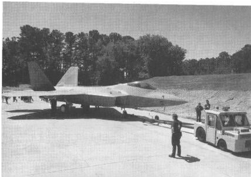
The F-22A Raptor is shorter in length and height than either the F-15C or YF-22A. Its wing span at 44 ft, 6 in is greater than either one. Today's Raptor is very similar in size to yesterday's Eagle. ( Lockheed Martin Corporation. )
