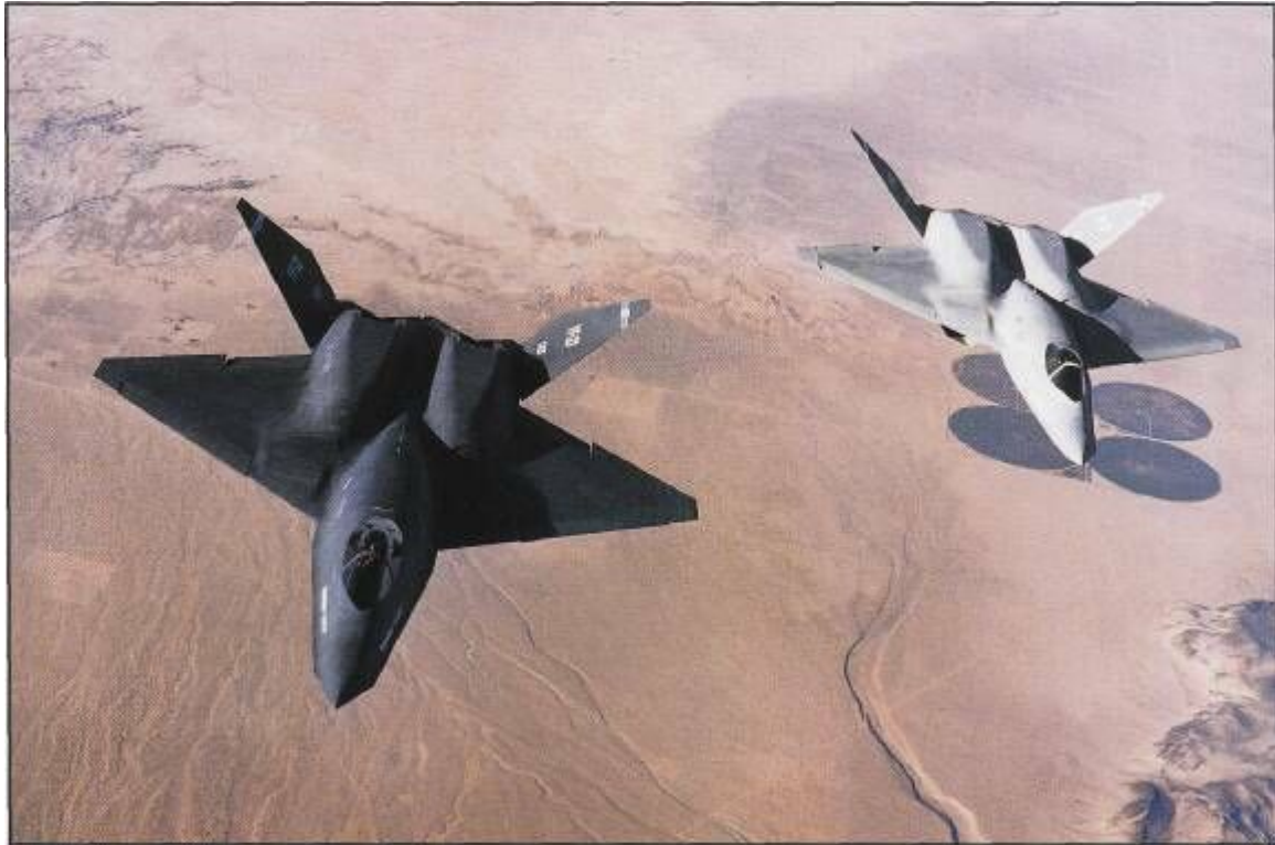
With their first flights respectively occurring on August 27 and October 26, 1990 at Edwards AFB, the two Northrop/McDonnell Douglas YF-23A ATF prototypes fly in formation, circa late 1990. First to fly, the black one (YF119-powered) was nicknamed the Black Widow II . Second to fly, the multihued light to medium gray one (YF-120-powered) was dubbed the Gray Ghost (U.S. Air Force.)
