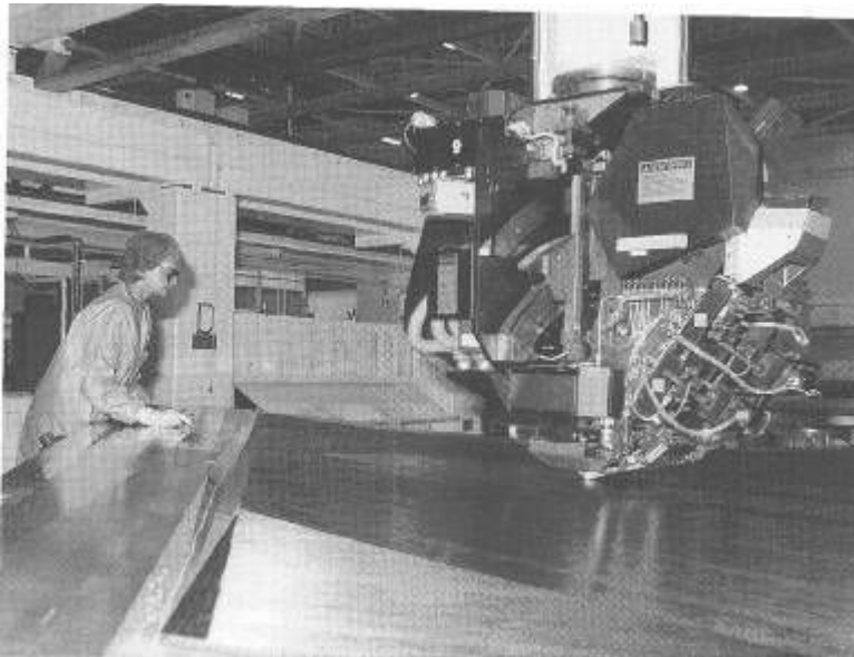
Boeing uses advanced processes to build wing skins for the F-22. Agnes Ulrich, Boeing plastic bench mechanic, monitors an automated contour tape-laying machine that applies layers of advanced composite resin-impregnated tape on top of a precisely curved surface to form a wing skin. Automated fabrication replaces the conventional and labor-intensive hand-layup method. ( The Boeing Company. )
