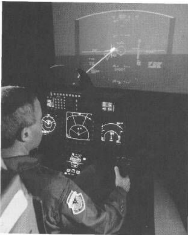
Another view of an F-22 cockpit simulator shows a pilot firing a missile launch at a target. Note right hand on control stick and thumb on fire button. (Lockheed Martin Corporation.)
