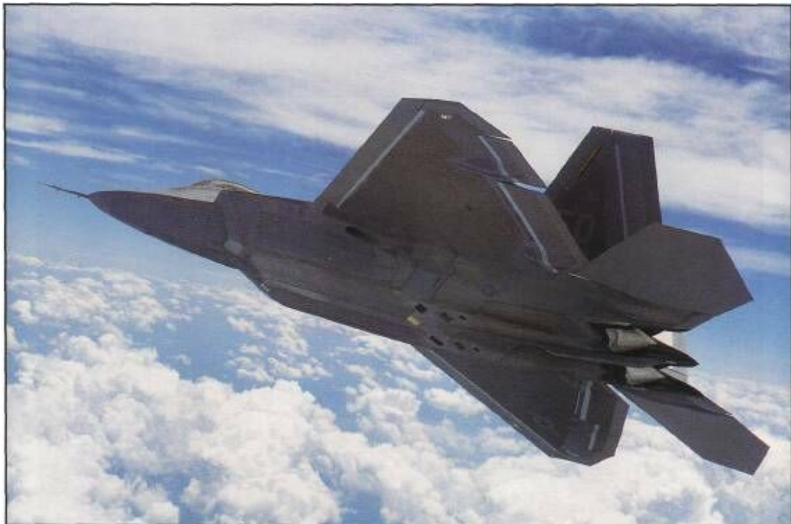
As it banks to the right, Raptor 02 (AF 91-0002) flies through cumulus and cirrus clouds. Using its afterburners, the F-22 is capable of more than Mach number 2 (Mn 2+) at altitude (Mn 1.5+ without afterburners) and Mn 1+ at sea level. ( Lockheed Martin Corporation. )
