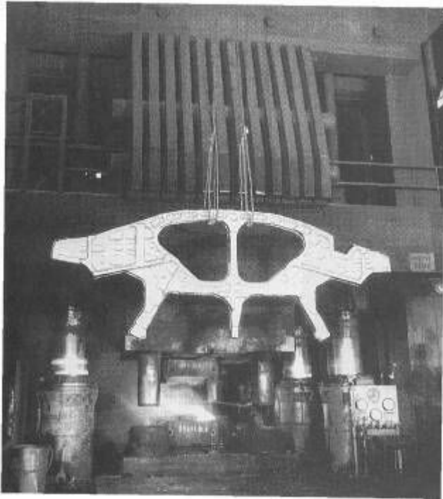
Manufactured by Wyman Gordon in North Grafton, Massachusetts, this midfuselage bulkhead is the world's largest titanium alloy forging. (Lockheed Martin Corporation.)
