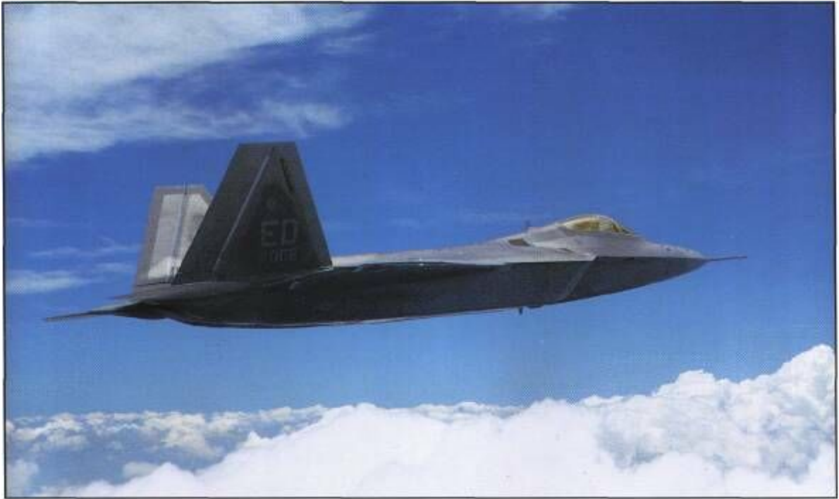
The F-22 features two wide-chord, large-area vertical tails with large-area rudders. Canted outward for stealth reasons, its vertical tails offer excellent low-, medium- and high-speed stability. The ED on the tail denotes Edwards AFB. ( Lockheed Martin Corporation. )
