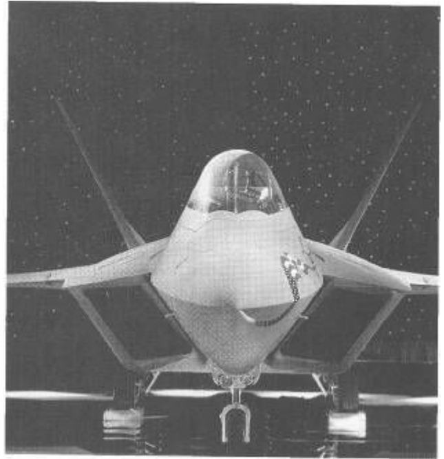
This head-on view of Raptor 01 during its rollout ceremony shows its deep, diamond-shaped fuselage to good advantage. Its very large engine air inlets are noteworthy. ( Lockheed Martin Corporation. )
