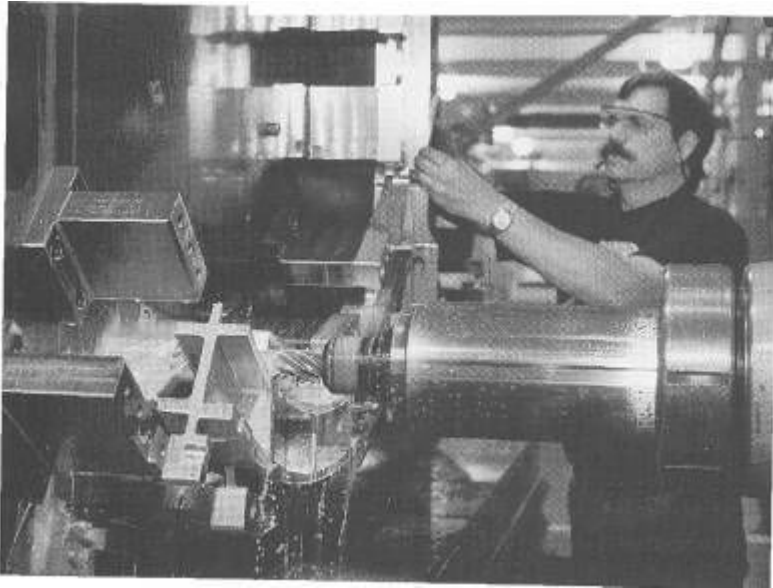
Machinist Mike Osborne, Boeing Defense and Space Group manufacturing, uses a horizontal-boring mill to cut part of an F-22 aft fuselage frame in February 1995. A week earlier, the air vehicle Critical Design Review, a major milestone, was completed. ( The Boeing Company. )
