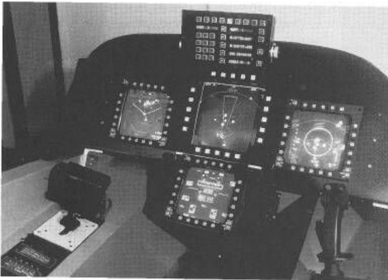
The Boeing-developed tactical displays for the F-22 are shown on this simulator. The defense display on the left gives pilots the information they need to protect themselves against threats. The situation display in the middle provides them with overall situation awareness and navigation information. The attack display on the right gives them the information necessary to attack a target. ( The Boeing Company. )
