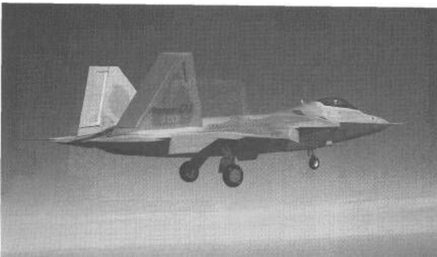
The Raptor's twin outward-canted vertical stabilizers are required for its stability at very high speeds. Although the F-22's maximum speed is classified, it probably matches the F-15C's announced maximum speed of Mn 2.5. ( F-22 Team. )
