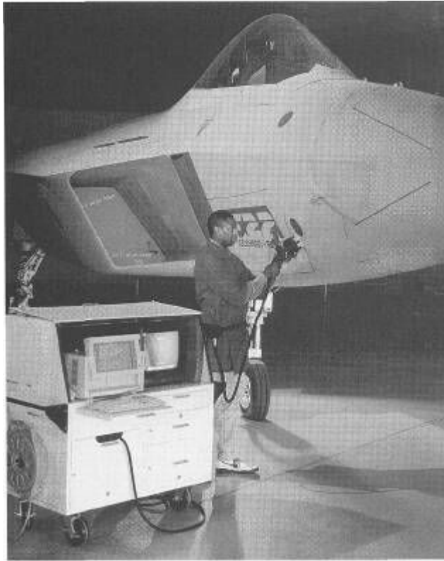
In a demonstration of a tool that will be very important in the assembly of F-22s, LMAS' Bryant McKee inspects the gap between the avionics bay access door and the forward fuselage of the YF-22A ATF prototype, circa early 1996. (Lockheed Martin Corporation.)
