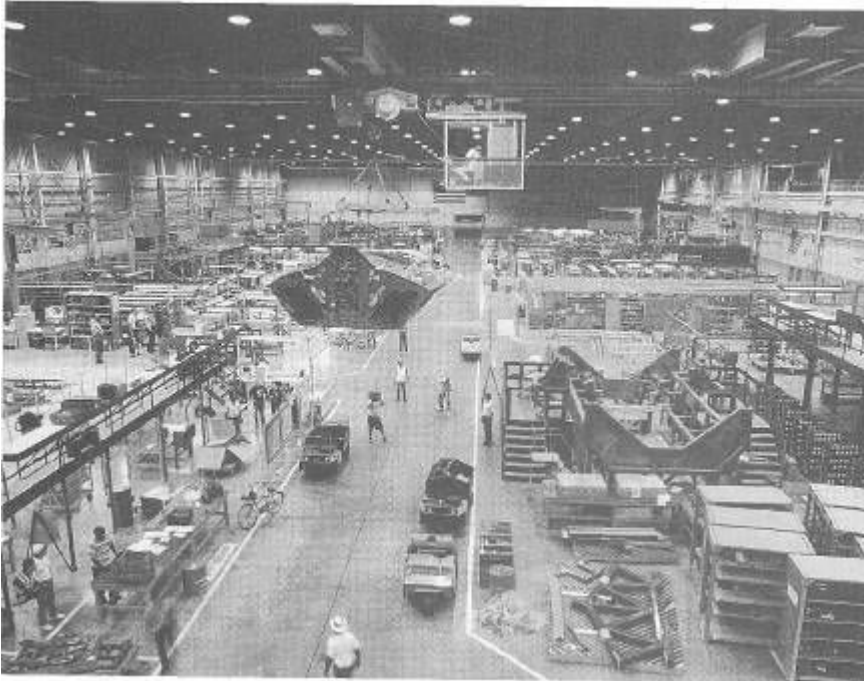
An F-22 midfuselage section moves toward its final assembly area. (Lockheed Martin Corporation.)
