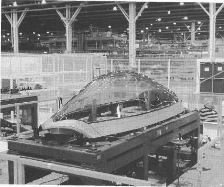
This is the first cockpit canopy for the first Raptor as it appeared in January 1996. It is approximately 140 in long and 45 in wide and weighs about 350 lb. ( Lockheed Martin Corporation. )
