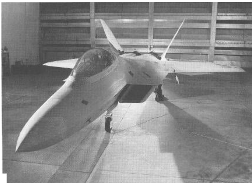
Enter the fifth-generation stealth aircraft, the first EMD F-22A Raptor, shown shortly after it received its multihued gray paint job and just before its public debut. As the F-22 is of about the same size and weight as the F-15C Eagle, its low observability makes it much more survivable than its forerunner. (Lockheed Martin Corporation.)
