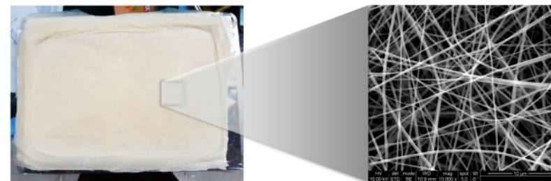
Polybenzimidazole nanofiber mats to increase the mechanical strength and reduce swelling of membranes.
