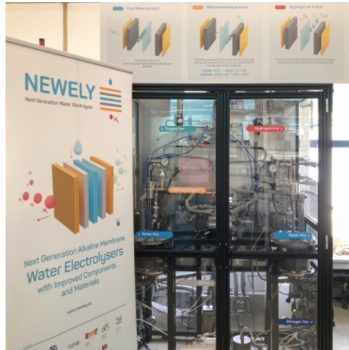
Test bench designed and constructed by FBK to test NEWELY materials.
