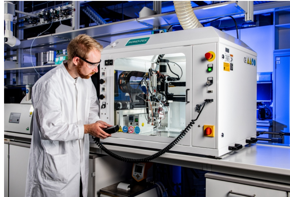
Automated electrode spray-coating
