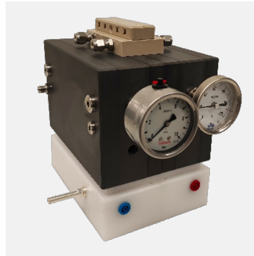
Single cell AEMWE testing device based on hydraulic cell compression
