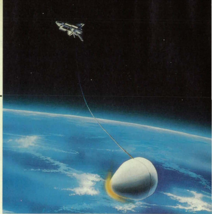
Sensor-embedded "smart" structures could play an important role in future space research projects such as the Shuttle Tethered Aerothermodynamic Research Facility (pictured above), which will study the interaction of the atmosphere with satellites at hypersonic speeds. Fiber optic sensors embedded in the tether would offer a cost-effective way to monitor the line's health and performance. See page 20. (Photo courtesy NASA)
