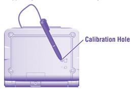
• To calibrate the stylus to the touch screen, insert the tip of the stylus into the **Calibration Hole** on the back of the handheld.
