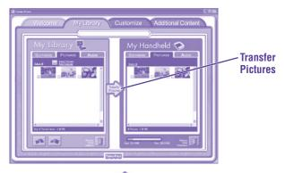
• Click on the **Transfer Pictures** button to move the pictures onto the **My Handheld** side of the screen and the handheld.
