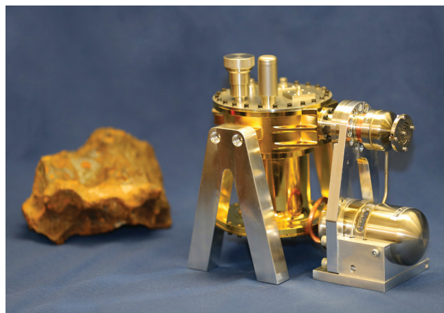
The GeMini Plus gamma-ray detector contains a high-purity germanium sensor enclosed by a temperature sealed housing (gold cylinder). The sensor is cooled to liquid nitrogen temperatures by a long-life cryocooler (silver cylinders) (Image credit: LLNL).
