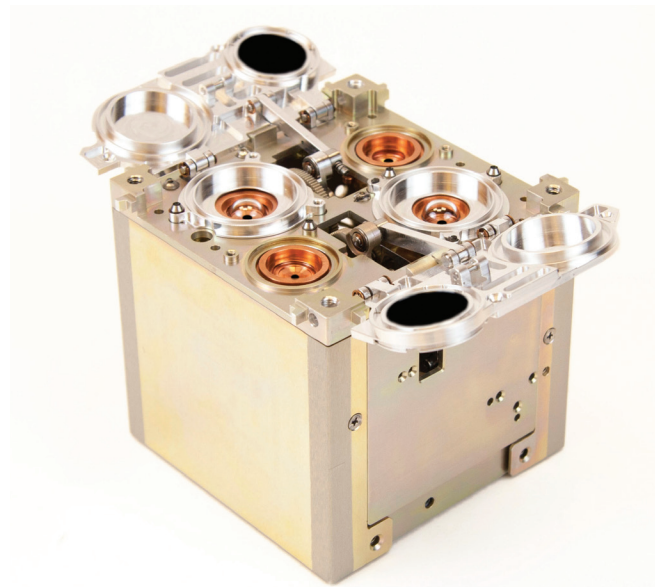
The RAVAN flight payload with covers open, showing the four radiometer sensors. (Image credit: JHU APL/L-1 Standards and Technology)
