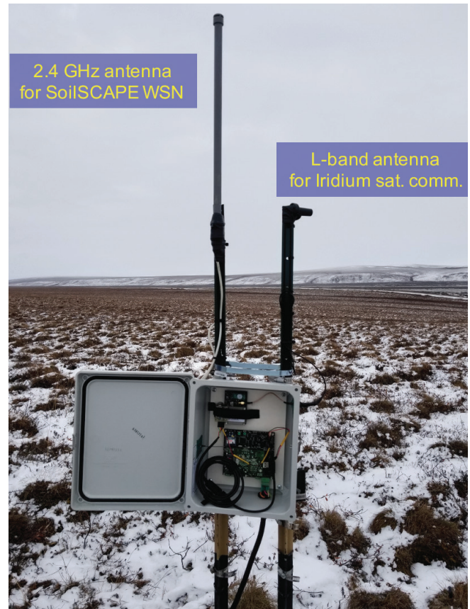
A SoilSCAPE base station (coordinator) at an Alaska site. The coordinator receives data from the SoilSCAPE probes (the wireless sensor network, or WSN) and sends it to the lab via satellite. The coordinator also receives commands from the lab and relays them to the SoilSCAPE sensors using the same communication path in reverse.
