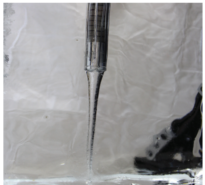
Laboratory prototype of a direct laser penetrator making its way through ice.
