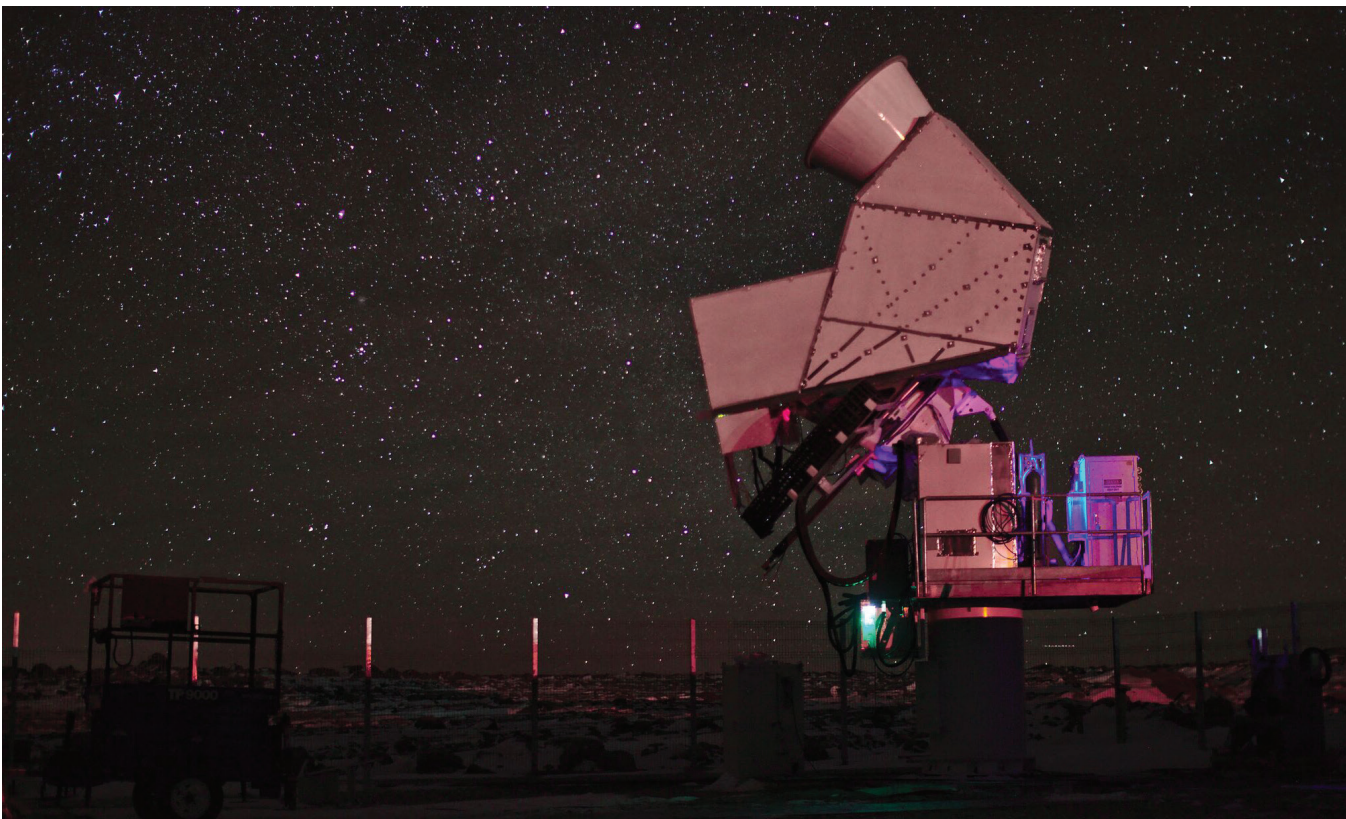
The 40 GHz CLASS telescope, shown at the site in Chile, has been taking science data since September 2016. A 90 GHz telescope is currently being deployed and prepared for commissioning.
