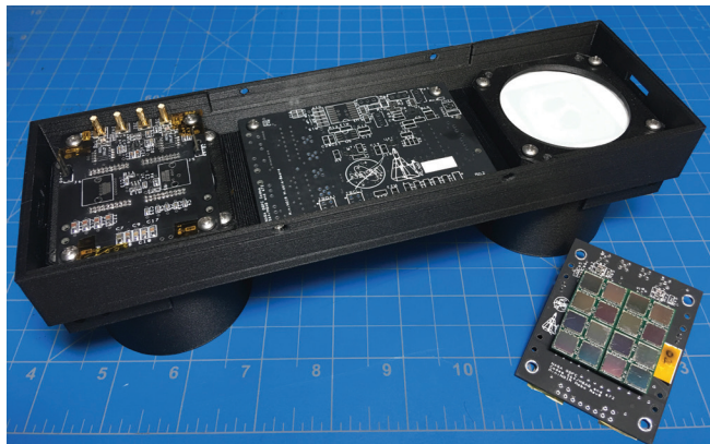
The INCA detector, showing the two scintillators, a bias voltage board, and SiPM arrays housed in the instrument frame.
