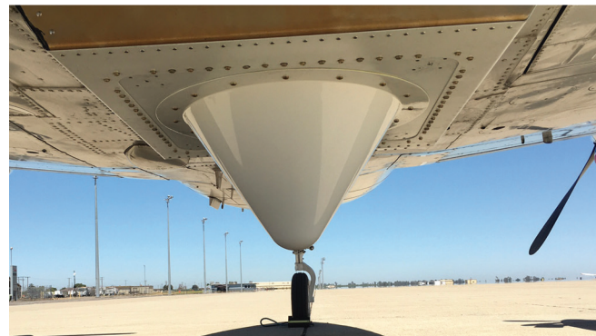
Top: The DopplerScatt team with the radar at JPL before aircraft installation. Bottom: DopplerScatt aboard King Air B200. (Image credit: NASA/JPL-Caltech)
