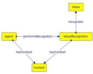
Figure 17 Value Recognition Schema
