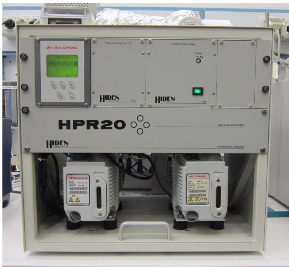
Figure 3. 15. A picture of the MS Hiden HPR-20 QIC.
