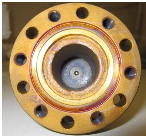
Figure 3. 4. Pictures of the FFC reactor. (a) represents the disposition of the upper part (b) inside the lower part (c) around which there is the electric heater.
