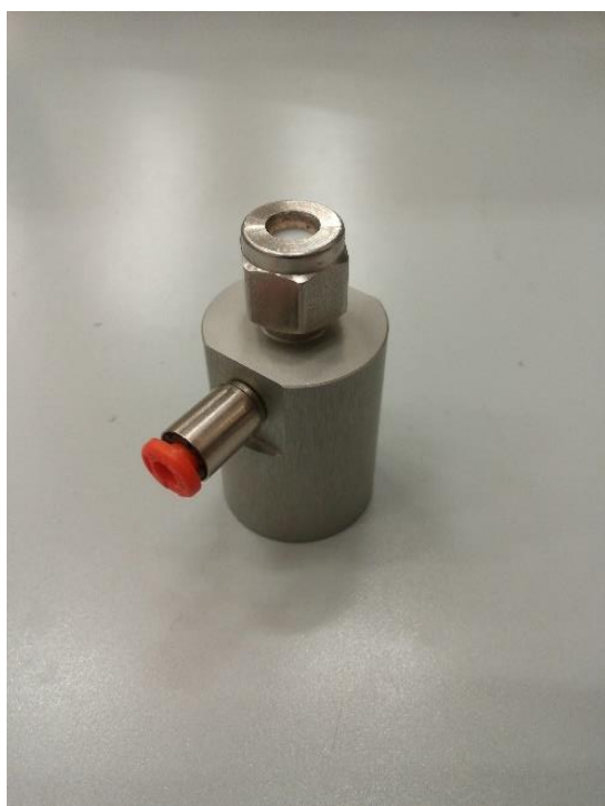
Figure 3. 10. Pictures of the connectors for the FF reactor. a. shows the connector for the LDPE tube on the left and the connector for the thermocouple on the top. b. shows the plastic O-ring used to seal the quartz tube with the connector.
