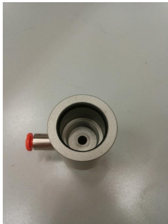
Figure 3. 10. Pictures of the connectors for the FF reactor. a. shows the connector for the LDPE tube on the left and the connector for the thermocouple on the top. b. shows the plastic O-ring used to seal the quartz tube with the connector.
