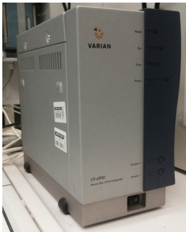
Figure 3. 13. A picture of the Varian microGC CP-4900.
