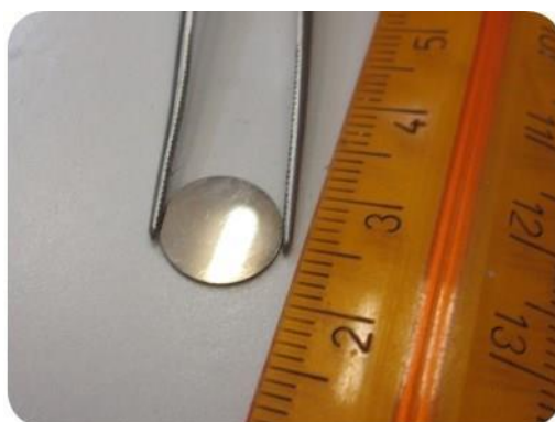
Figure 3. 3. A picture of the tested platinum catalyst.
