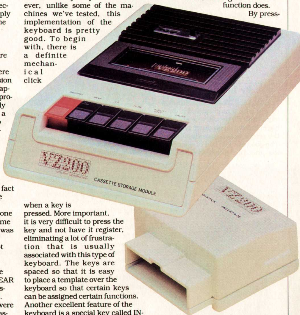
Peripherals for the VZ 200 include the cassette drive and joystick interface pictured above.
