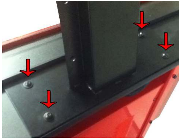
Step 2 - Secure Mounting Plate to Cabinet
