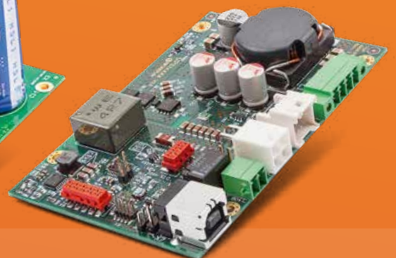
UPSI DC UPS CONTROL UNIT
