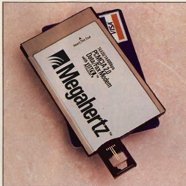
The Megahertz XJ1144's patented XJACK phone connector makes it one of the most portable modem solutions available.
