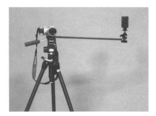
Fig. 4 Sony DSC-F707 on tripod with extension arm to support oblique IR light source.
