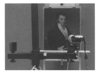
Fig. 3 Sony DSC-F707, 5 Mp Digital Camera on camera stand, with opposed IR light source (Sony Model #HVL-IRC).
