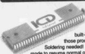
100% Compatible, plug-in replacement 14.3MHz 68000 processor for use with any Amiga 500,1000, 1500 or 2000. Incorporates a special built-in 32K RAM cache to speed up those processor-intensive operations. No Soldering needed! Also features a 7MHz fall-back mode to resume normal operating speed, when required.
