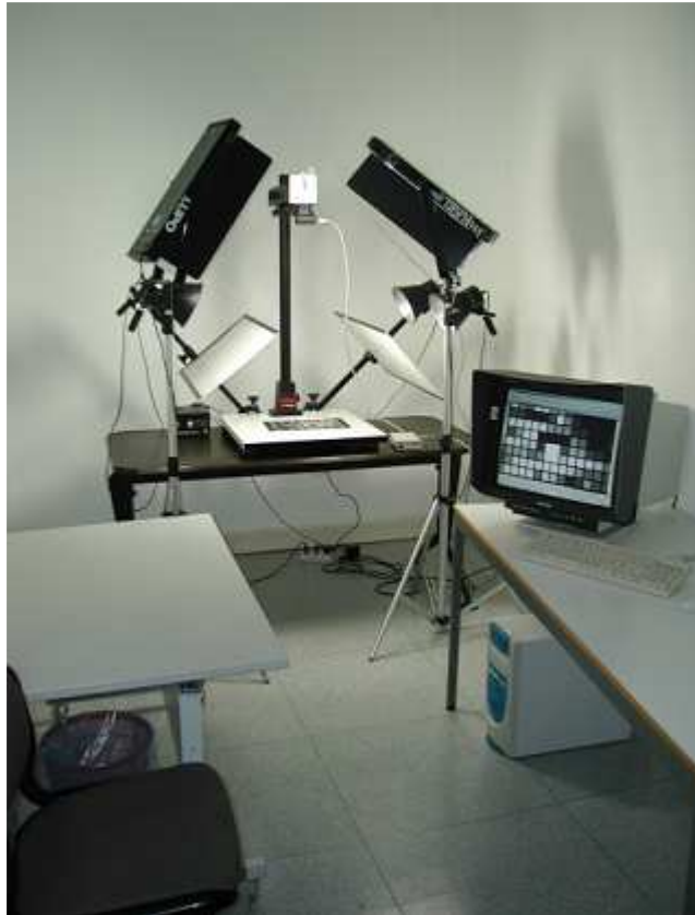
Fig. 2 – A shot of our acquisition system. It can be mounted on a tripod but also hanged from above using a simple frame like this one
