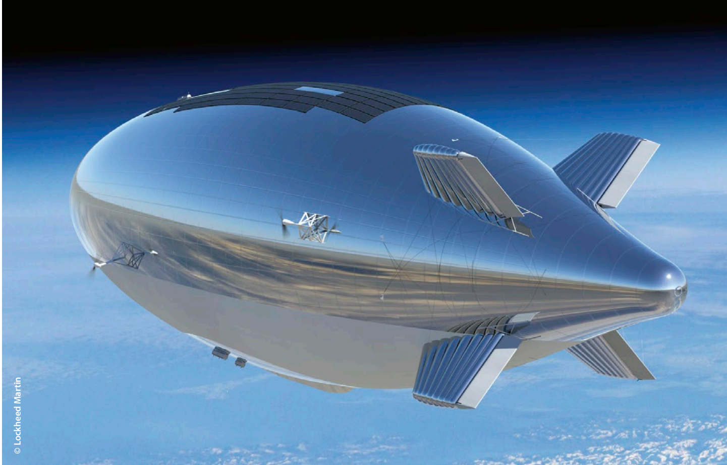
Figure 4: Example of a HAPS LTA: ISIS (Integrated Sensor is Structure) was a joint Defence Advanced Research Projects Agency (DARPA) and US Air Force Science and Technology (S&T) programme. 10
