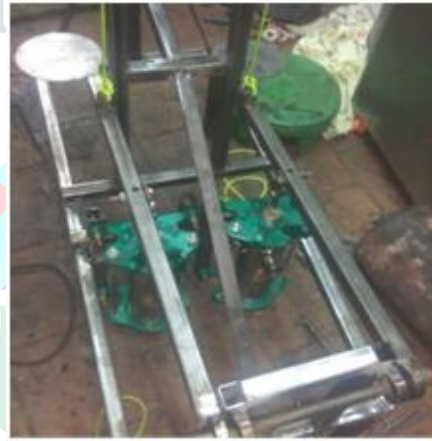
Figure 2: Cylinders connected to treadles
