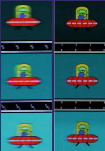
Turning on backlight strobing blur reduction (right) greatly increases image clarity for fast motion
