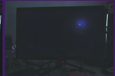
Without local dimming normal LCD monitors leak too much light to produce meaningful HDR, but full array local dimming backlights can illuminate only the backlight zones that are needed (images edited to exaggerate the effect)
