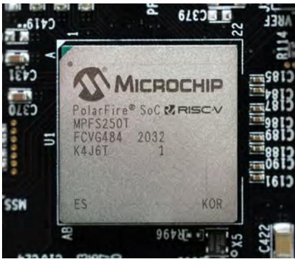
The SoC at the heart of the board offers surprisingly robust performance, plus plenty of room for FPGA gateware
