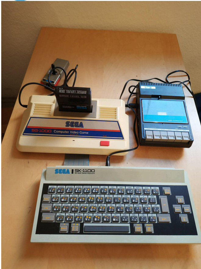
Fig. 11 - The optional SK-1100 keyboard for the console, to which an additional tape player is also connected, to turn the SG-1000 into a home computer (source: Wikimedia - author: Darktrym)
