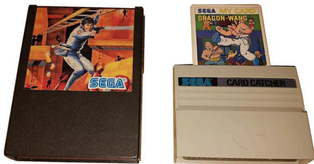
Fig. 6 - On the left is a ROM cartridge and, on the right, the Card Catcher adapter with a My Card (source: Wikimedia - author: Darktrym)
