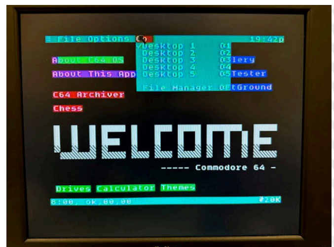
Fig. 5 - The GO menu with options to access the different desktops where to open applications
