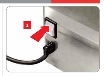
**2** Connect the machine by turning the main switch ON and simultaneously pressing down on the key .
