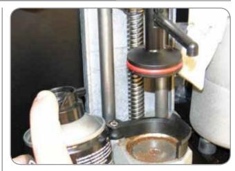
3 Move up the group by pressing the arrow up button and lubricate with Teflon spray the two bushes on bottom of the group.
