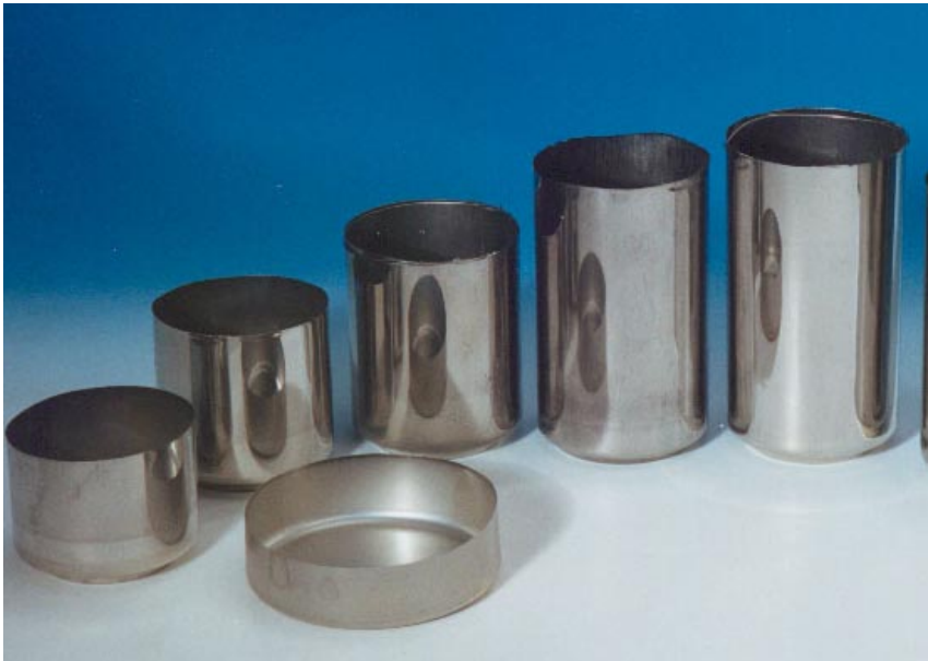
Figure 19 The drawn and ironed tinplate can: stages of manufacture
