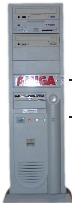
The EZTower is a bit of a beast! Here you can see the 6.5.25" bays and Martin's home-made floppy drive face plate..
