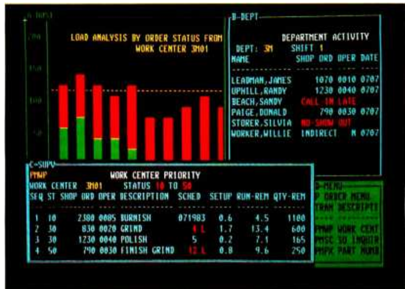
Photo 1: A shared screen on the new IBM 3270 PC. Four host programs can run at one time.
