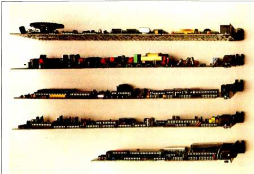
Photo 1: The thickness of the board configured with a speaker may concern you if you own an XT. From the top: Hayes, Microcom, Novation, Bizcomp, and Cermetek.
