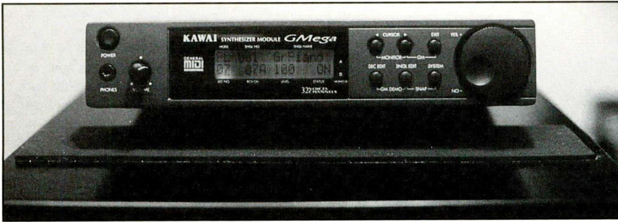
Kawai's GMega synth module can accommodate up to 32 MIDI channels simultaneously, has excellent drum sounds and offers lots of user-programmable patch options.
