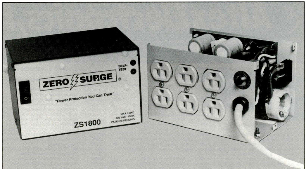
Zero Surge's Model ZS1800 surge/spike protector provides fast suppression of power-line surges without relying on traditional MOVs. It handles loads of up to 15 amperes at 117 volts ac.
