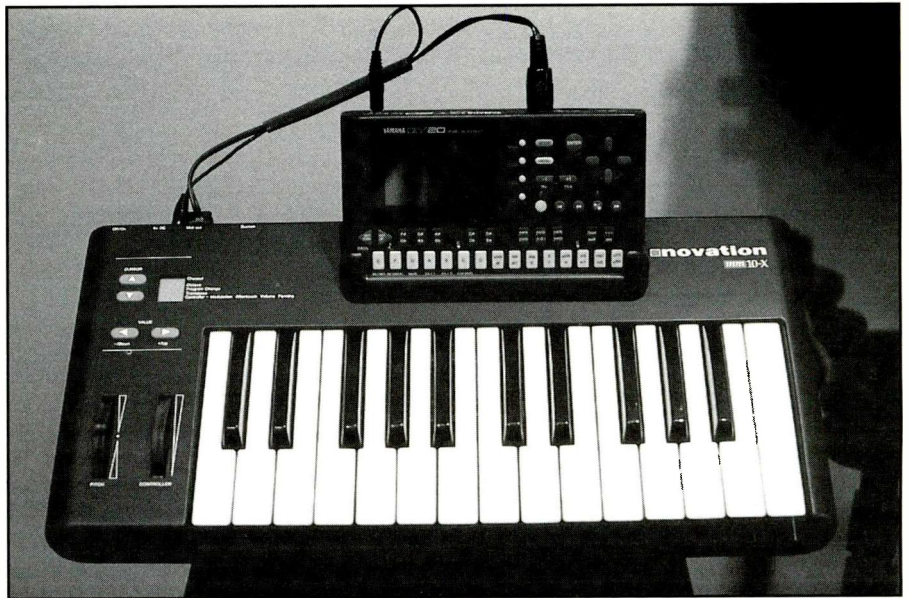
Novation's MM-10X MIDI keyboard controller shown with a Yamaha QY20 inserted and coupled to it—a marriage made in MIDI heaven—has a long list of sought-after features and, like the QY20, is portable.
