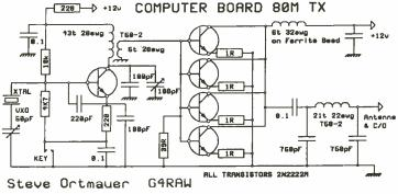
You will note the wire gauges are stated in SWG which are about one size smaller than AWG sizes. However, using the same gauge sizes in AWG will work just fine. Any of the given wire sizes can vary by as much as two sizes and still work without problem.
