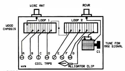
**FIGURE 3**— Pictorial representation of the figure 2 tuner circuit. A wooden base is used for the chassis. Loop 1 and Loop 2 can be affixed to the base with globs of sealant, such as Goop or silastic bathtub sealer. A rotary tap switch may be used as an alternative to the clip lead and screws for changing the inductance.
