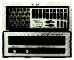
Top: Regency WHAMO-10, programmed using metal combs. Bottom: Tennelec MS-2, programmed using binary codes entered through the 0 and 1 keys (photo by Pam Parnass N9HRZ)
