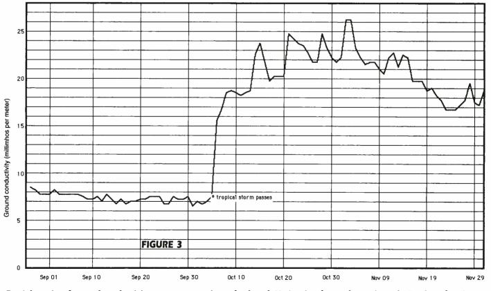
Partial results of ground conductivity measurements in my backyard. Notice the abrupt change in early October after the heavy rainfall associated with the tropical storm. Periodic heavy rainfall throughout the following month was responsible for maintaining the ground conductivity at a high level.
