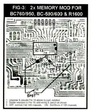
isolated, not touching anything. Slip a sewing needle between Pins 18 and 19 (if you're right-handed) or between Pins 19 and 20 (if you are left-handed). Angle the needle so that it uses the adjacent pin as a fulcrum and exerts a bit of upward force on Pin 19. Gently now! Very gentle.....
