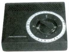
The same map used on the indicator board was cut out to retain only the circular bearing chart. This piece was cemented to the top of this Radio Shack rotator control box.
