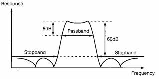
FIGURE 7: Response of a typical filter
