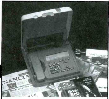
Y2k emergency communications associated with the power grid will be by landline telephone and via satellite using the MSAT system (pictured).
