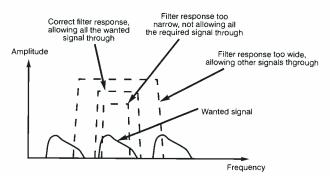
FIGURE 3: Choosing the correct filter bandwidth
