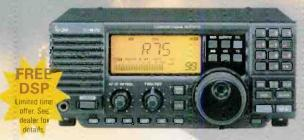
IC-R75 Pull out the weak signals. Cutting edge technology for today's serious DX listener, yet easy and affordable for a casual listener. 0.03 –60.0 MHz'; commercial grade; all mode; synchronous AM detection (S-AM); optional DSP; triple conversion; auto notch filter; twin passband tuning (PBT); large front mounted speaker; large display; well spaced keys and dials; 1000 memory channels; up to two optional filters; PC remote control with ICOM software for Windows®.
