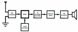
FIGURE 1: Block diagram of a single conversion superhet
