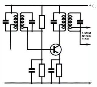
FIGURE 4: A circuit using an Interstage tuned transformer
