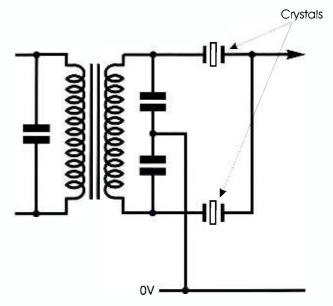
FIGURE 5: A basic crystal filter circuit
