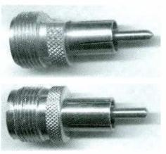
FIGURE 2. Female UHF to Motorola plug adaptor modified to fit BC248CLT (top). Unmodified adaptor (bottom)
