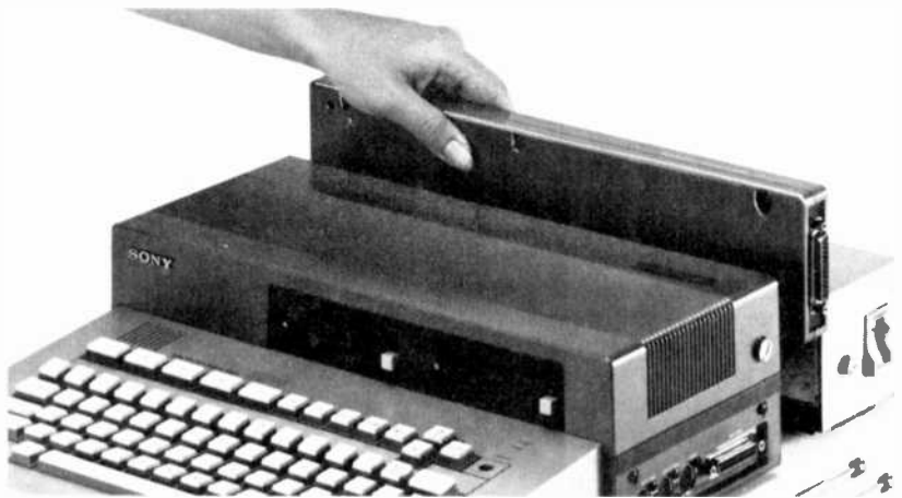
Expansion modules are installed between the main unit and power supply.
