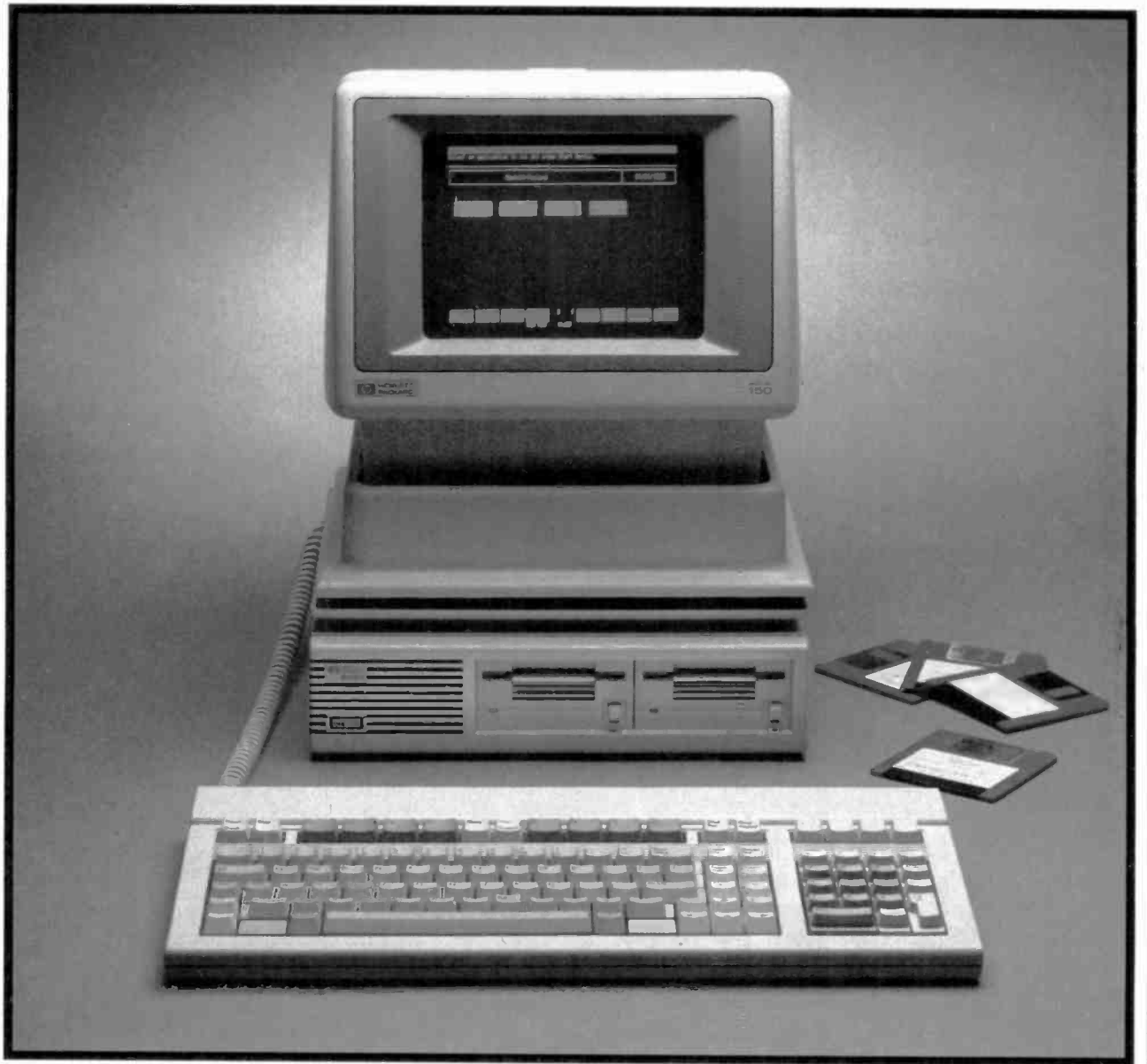
The unit has an extremely small footprint. Floppy disks at right are only 3½".
