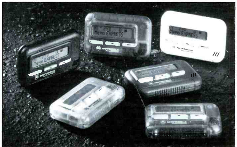
Alpha pagers, like these Motorola Memo Express units, are sophisticated devices that can deliver messages consisting of complete texts.
