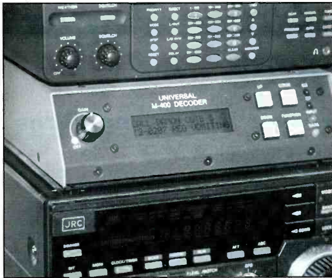
◀ The Universal M-400 Decoder connects to a scanner and reads out the text of the most commonly used digital pager modes.
