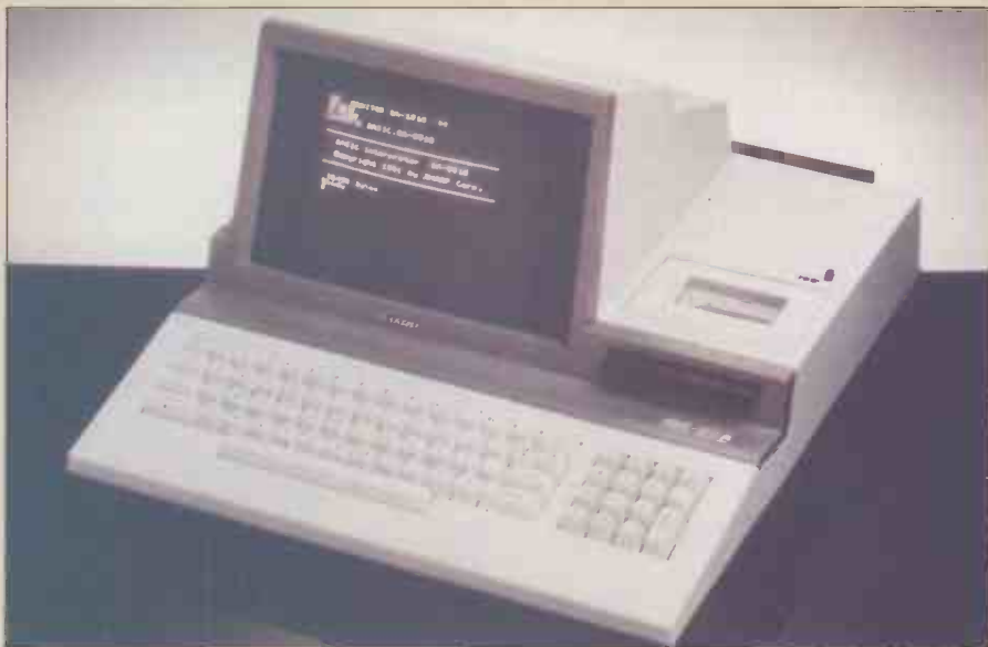
The MZ-80A's big selling point: a double size memory area devoted to the screen.
