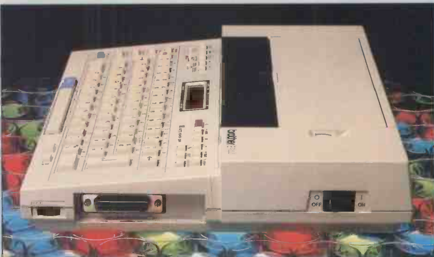
The RS232C port enables the machine to be used as a serial printer
