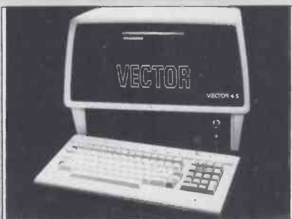
The Vector 4-S dual processor business micro has an automatic shift feature which detects different disk formats.
