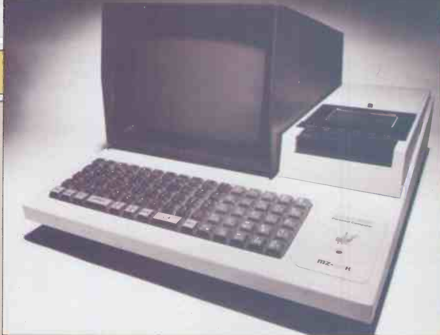
Cramped and unergonomic keyboard on the MZ-80K
