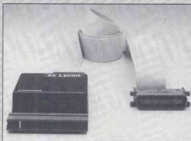
It may look like a cable with a big plug on one end: it is actually a peripheral for the Spectrum, intelligent enough to take the contents of the screen, and print them on a wide range of ordinary matrix printers. Price, including a Centronics cable, is £45. It also prints, normally. ZX Lprint III is available from Euroelectronics at 26 Clarence Square, Cheltenham, Gloucester. Phone (0242) 582009.
