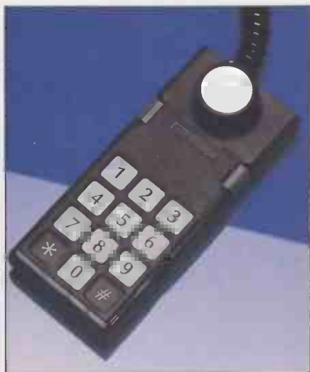
The joystick acts as a numeric keypad
