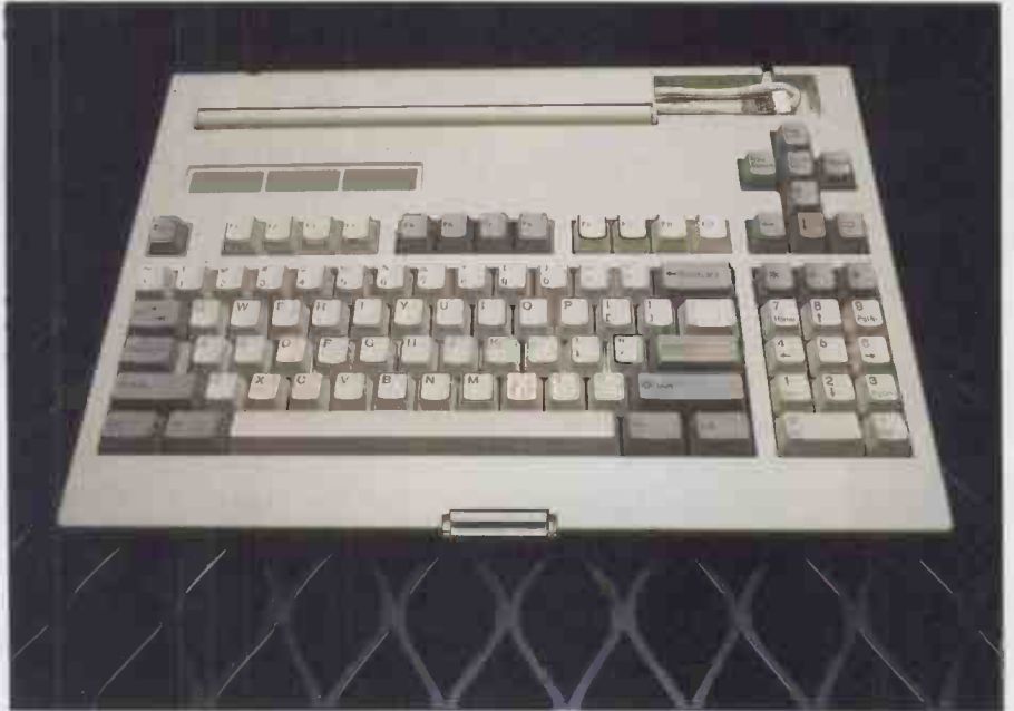
The keyboard takes up an unusual amount of desk space. The cursor key cluster sits in a curious position above the numeric keypad
