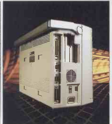
Four blanking plates can be seen, but the NEC uses three expansion cards
