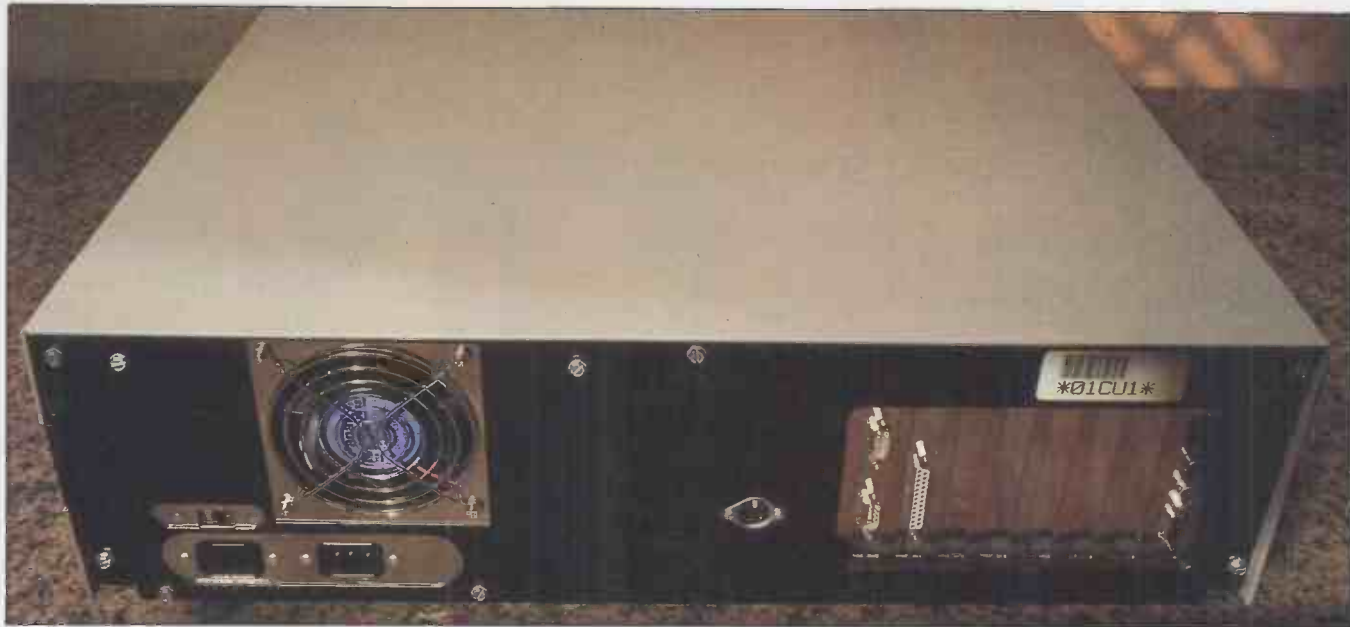
The serial and parallel ports are accessed from two openings which do not link to the six internal expansion slots
