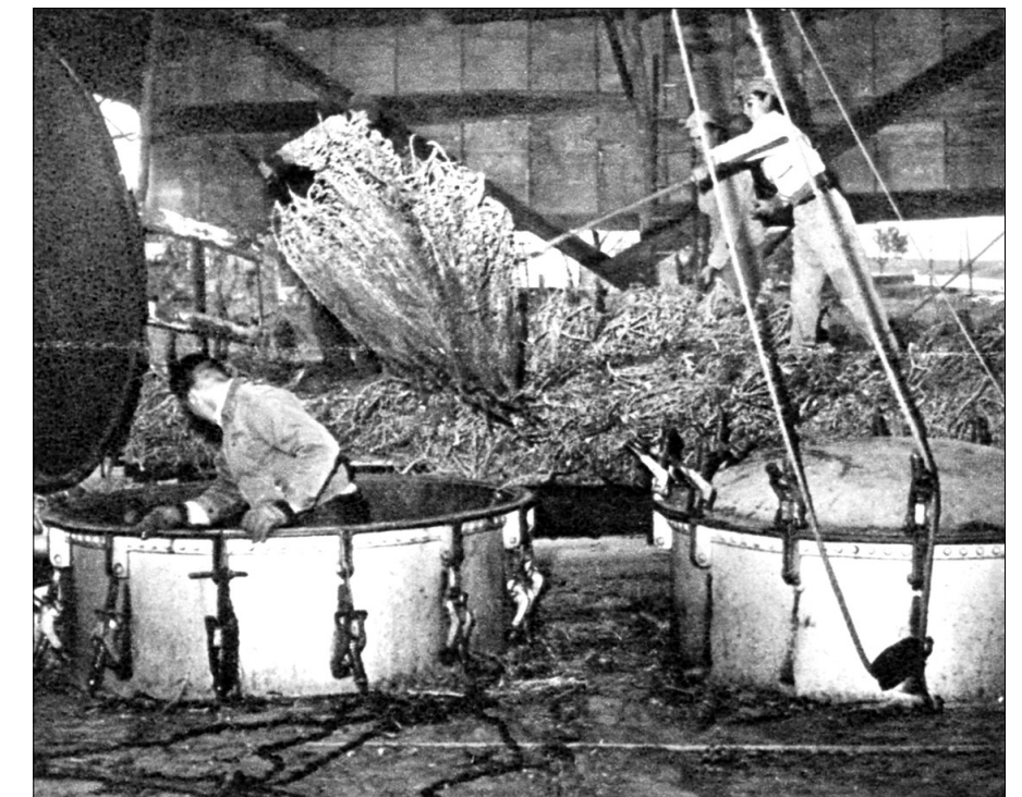
Loading and stomping down wormseed plants in still kettles, 1963. Photograph by A. Aubrey Bodine. (Copyright Jennifer B. Bodine. Courtesy of www.aubreybodine.com.)
