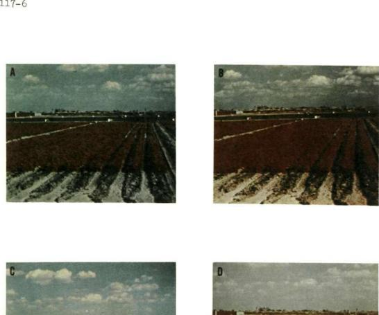
Figure 1.- Representative prints obtained by processing Kodak Ektachrome Infrared Aero, type 8443, and Kodak Aerochrome, type 2443, films to both positives and negatives. Print A is from a positive transparency of 8443, print B is from a negative transparency of 8443, print C is from a positive transparency of 2443, and print D is from a negative transparency of 2443 film.
